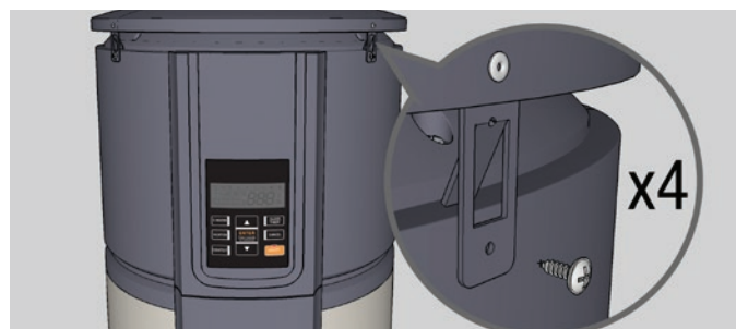
Fix rain cover into position using suitable screws (4 locations)
